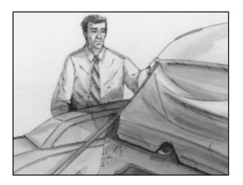
5. Pull the boot center cover from behind the rear seatback and place it over the inner sides of the boot side covers and the lowered top.
